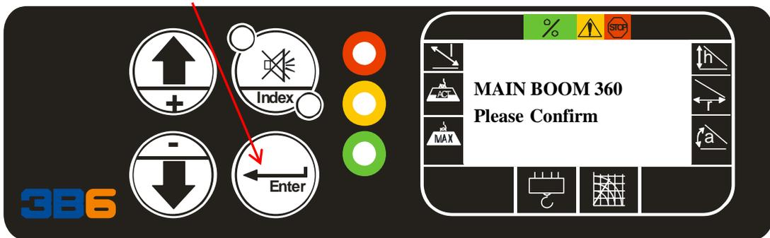
If the machine has a winch, you will have to press and release the ENTER pushbutton again to confirm the parts of line.
