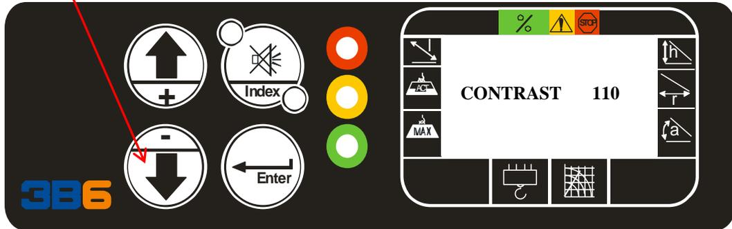
Press and release the DOWN pushbutton 4-5 more times and the screen values should appear.
