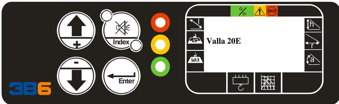
Now press and release the ENTER pushbutton to confirm the operating mode. You may have to press and release the ENTER pushbutton one time.
