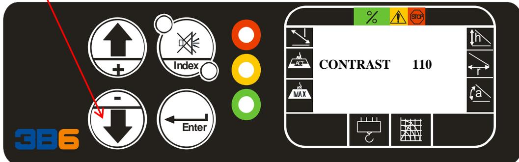
Once you have adjusted the value to see the screen 100-120 is normal. The display will automatically save the changes. If you recycle the power and the screen is blank again and the value you set is not saved. The Battery PCB may have an issue and require repaired.
