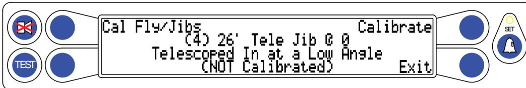
6. Press the **Calibrate** button and the system will ask for the corrected radius for this configuration. Measure the current radius and enter in feet and tenths of a foot. Press the **Exit** button.
