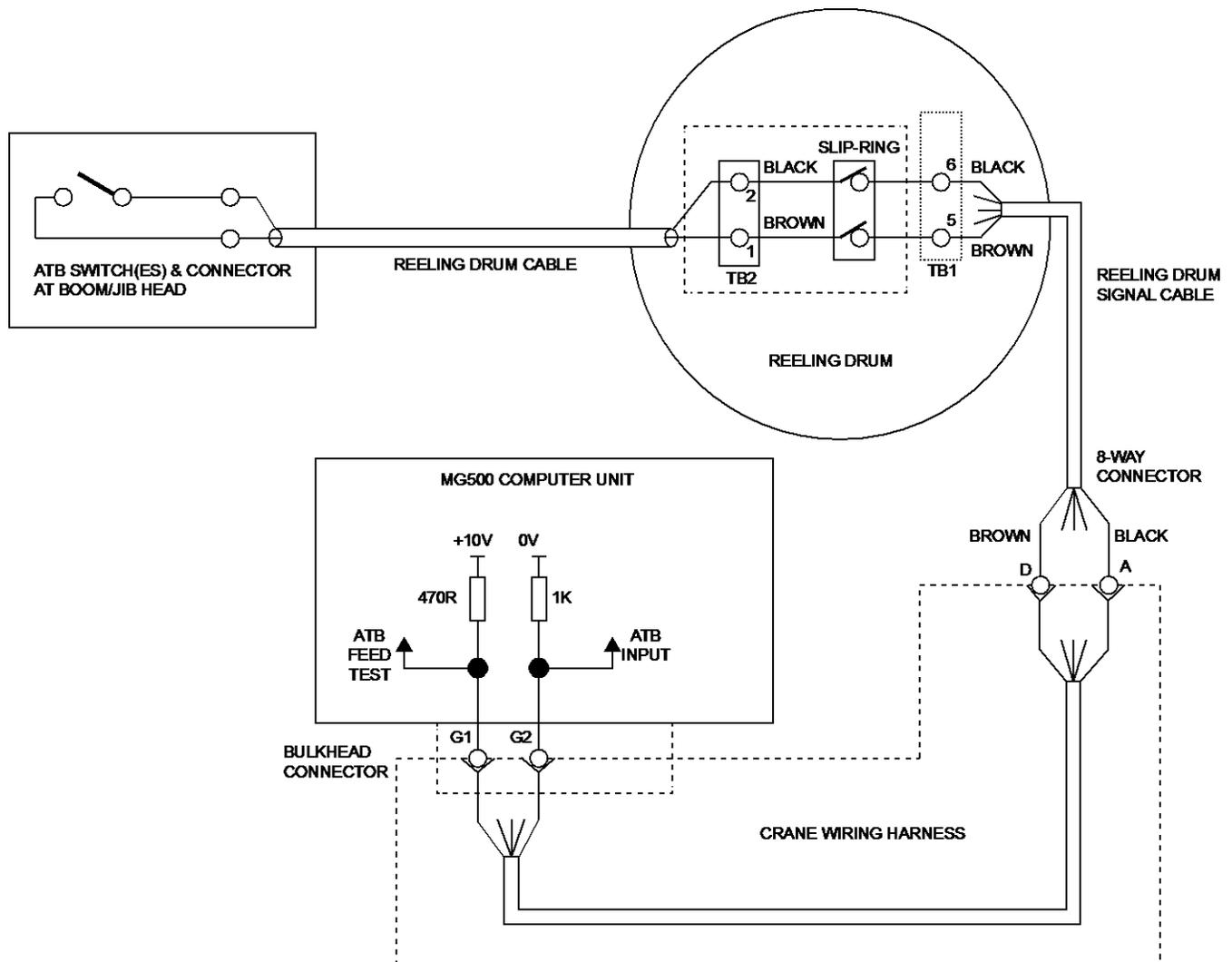
FIGURE 5.8 ANTI-TWO-BLOCK FUNCTION SCHEMATIC
