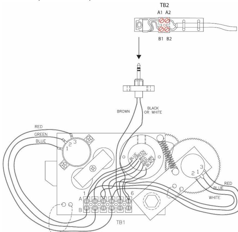
FIGURE 5.8.2 - CHECKING THE ANTI-TWO-BLOCK CIRCUIT
