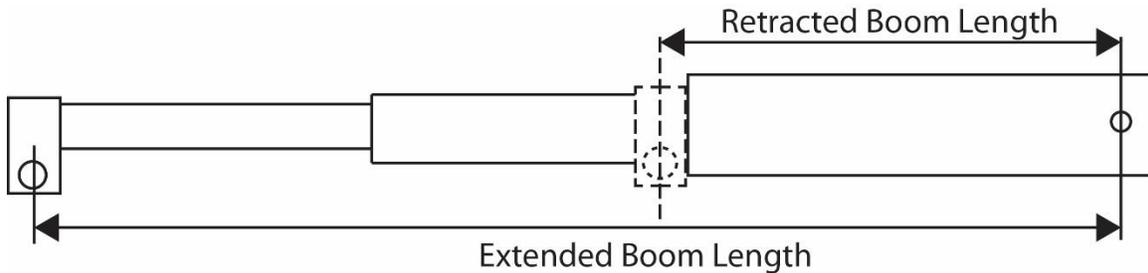
$$\text{Extended Length} - \text{Retracted Length} = \text{Span}$$
