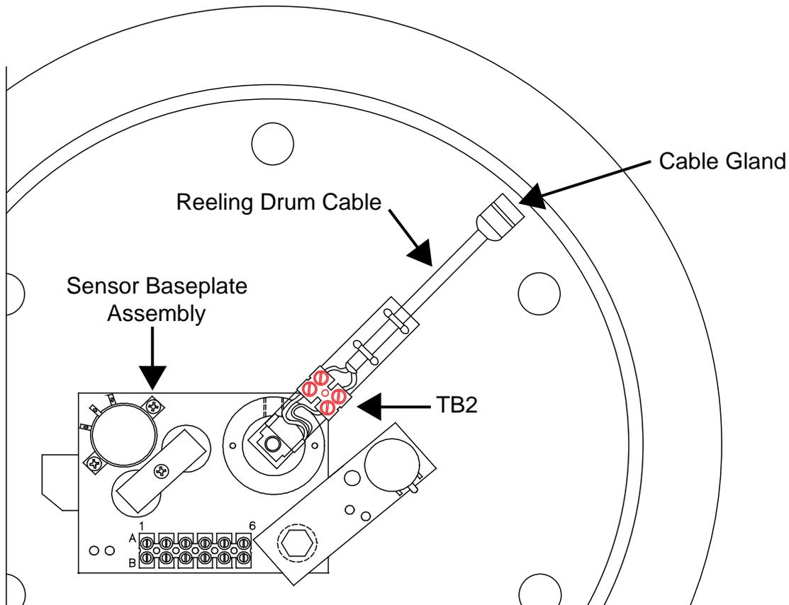
FIGURE 5.7.9 REELING DRUM CABLE CONNECTION ON THE REELING DRUM
