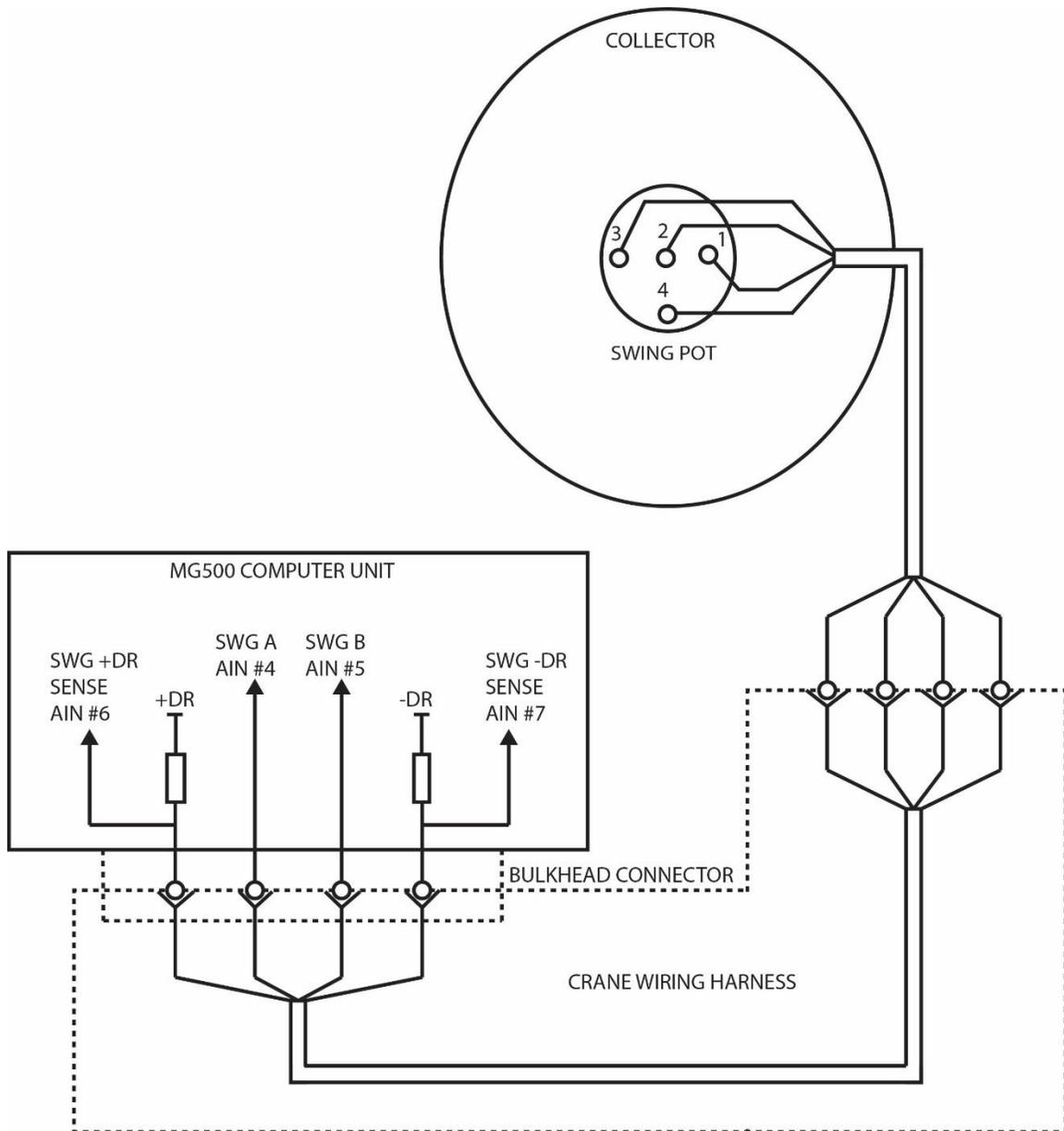
FIGURE 5.9 - SWING SENSOR SCHEMATIC
