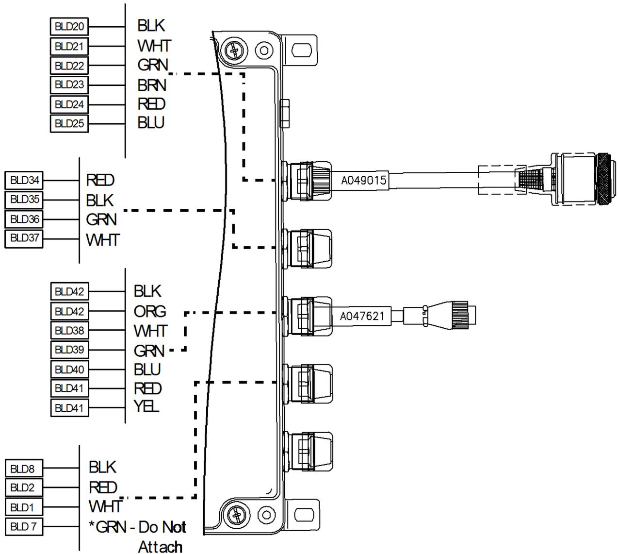
**\*NOTE:** The Green wire may have been replaced by a jumper wire inside the MG400 computer from B+ to Relay 2 C. In this case, use a jumper wire from BLD 3 to BLD 7.
