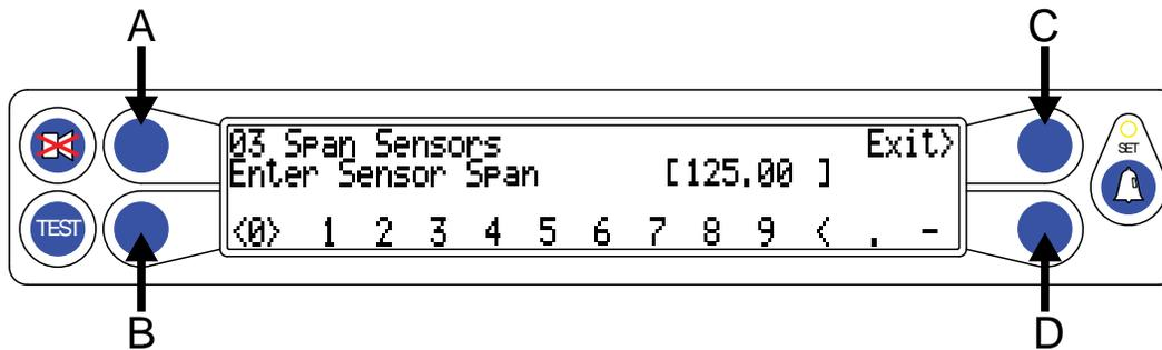
Use the **B** and **D** buttons to scroll left and right. The “cursor” will appear as flashing < > brackets on either side of the number. Use the **A** button to enter the number. Use the **C** button to exit the number entry subroutine.
