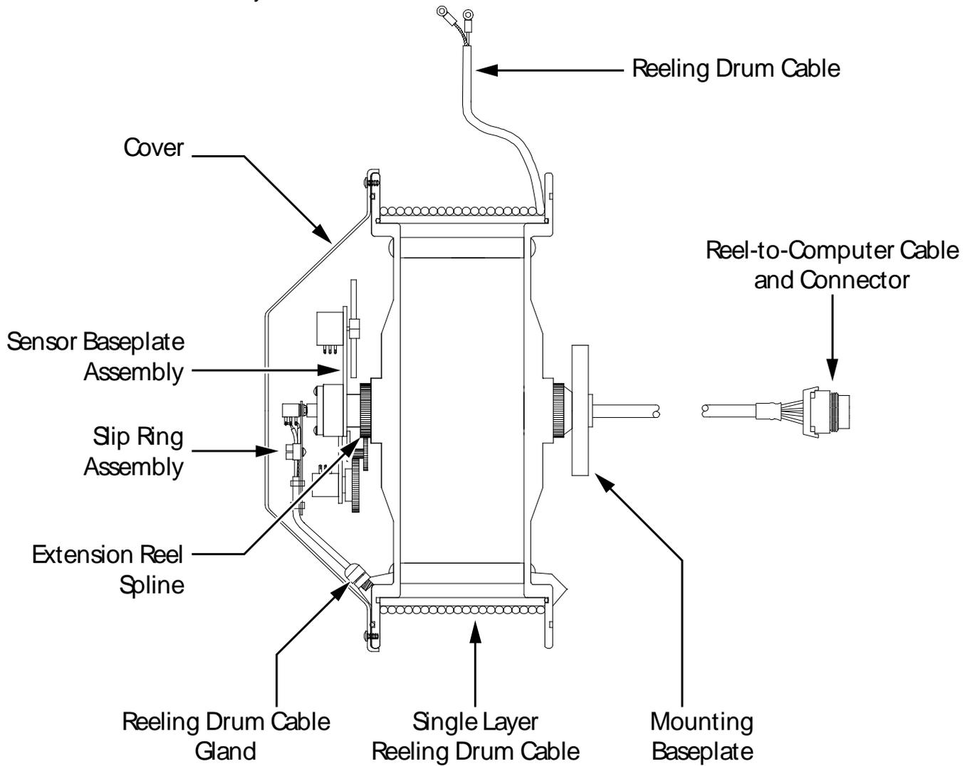
FIGURE 5.7 – REELING DRUM CUT-AWAY DRAWING
