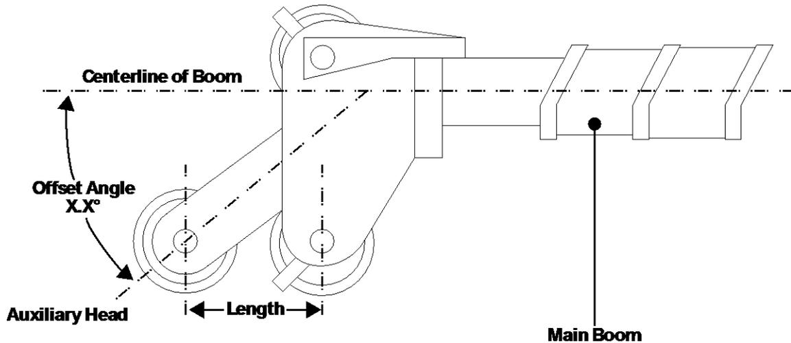
**Length** - Measure the distance between the Auxiliary Head sheave and the Main Head sheave.
